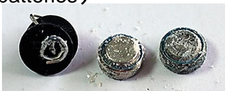
<Leakage by long-term use>
